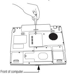
(Sample Illustration) Unscrewing the memory module slot cover
